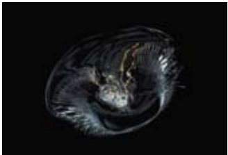
Bull's eye chip up to 5 mm diameter
