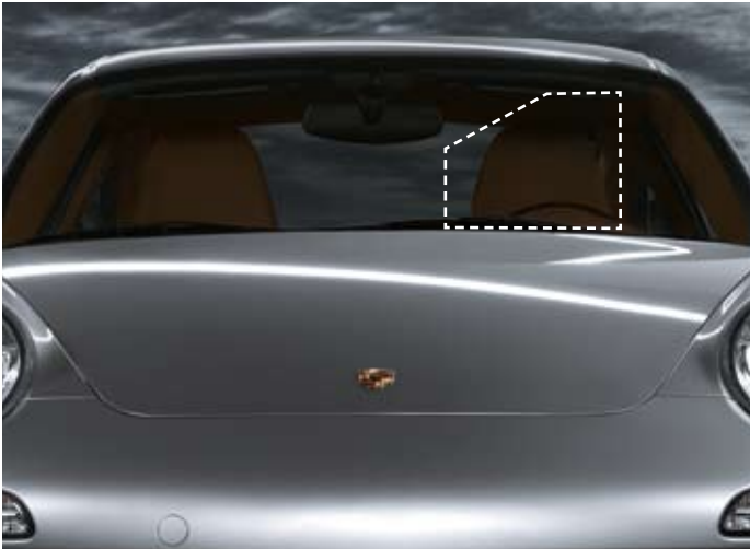
For safety reasons, glass cannot be repaired in the area marked
