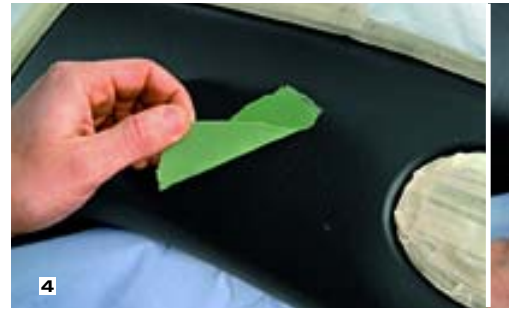
4 The dried mould film is removed carefully after about five minutes.
