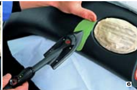
5 After removing raised parts with fine emery paper, Henrik fills the hollows with B Compound. 6 The surface pattern is copied onto the B Compound with the heat sealing iron. 7 The heat sealing iron can be adjusted in a range from approx. 50° C to 220° C.
