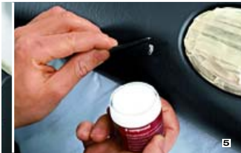
5 After removing raised parts with fine emery paper, Henrik fills the hollows with B Compound. 6 The surface pattern is copied onto the B Compound with the heat sealing iron. 7 The heat sealing iron can be adjusted in a range from approx. 50° C to 220° C.
