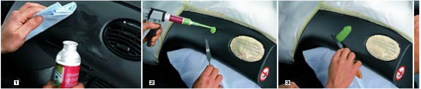
1 Careful cleaning of the whole area. 2 After the cut-out area is defined by masking paper and tape, the green mouldmaker is applied evenly using the gun. 3 Spreading with the palette knife to achieve a thin film.
