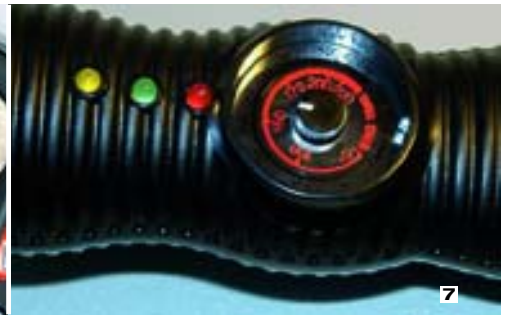
5 After removing raised parts with fine emery paper, Henrik fills the hollows with B Compound. 6 The surface pattern is copied onto the B Compound with the heat sealing iron. 7 The heat sealing iron can be adjusted in a range from approx. 50° C to 220° C.
