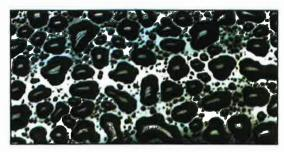
Fig. 16 Xzilon Green at 500 hours (detail)
