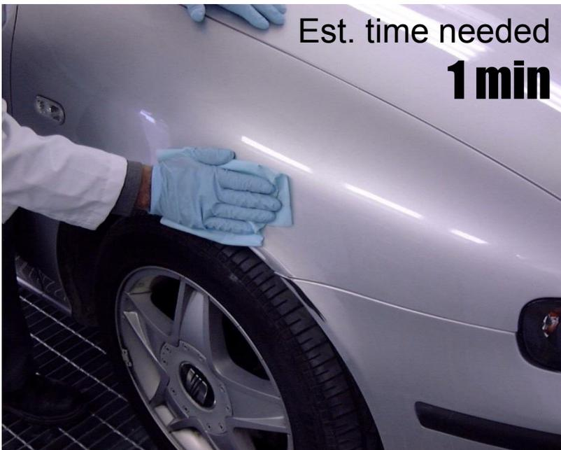
Degrease to eliminate impurities using
