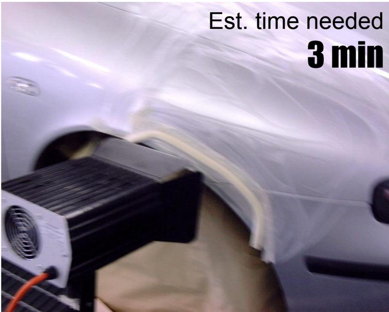
Expose to the UV lamp rays for 3-4 min depending on the thickness
