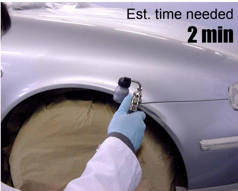
Apply the water based base coat
