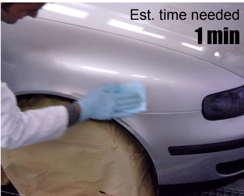
Degrease to eliminate impurities using Silicone remover
