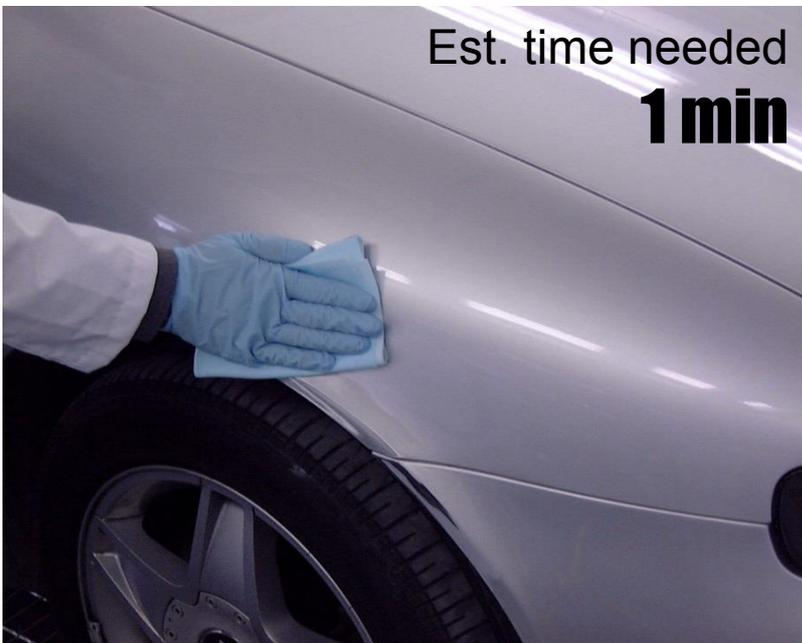
Degrease to eliminate impurities using Silicone remover
