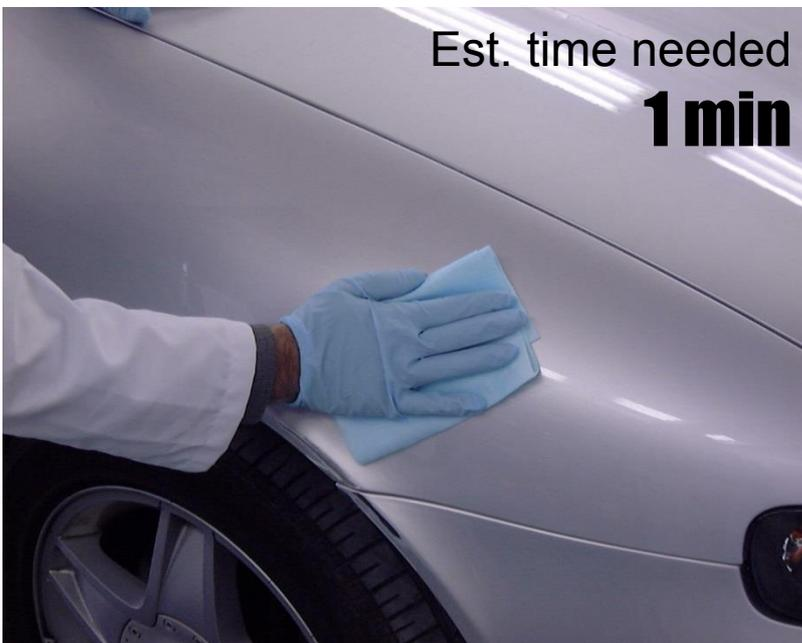
Degrease to eliminate impurities using Silicone remover
