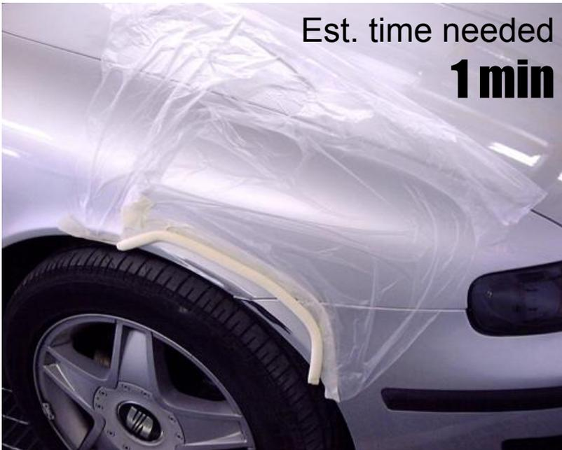
Mask the surface to be treated with the primer (L19008)
