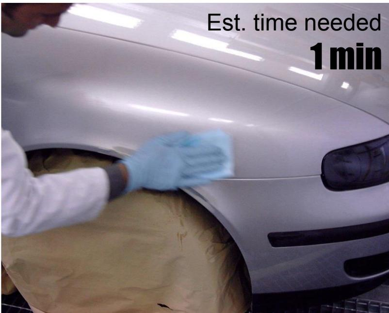
Degrease to eliminate impurities using Silicone remover
