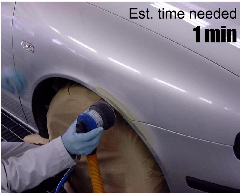
Sand the surface (treated with the UV-A1 Primer) with P400
