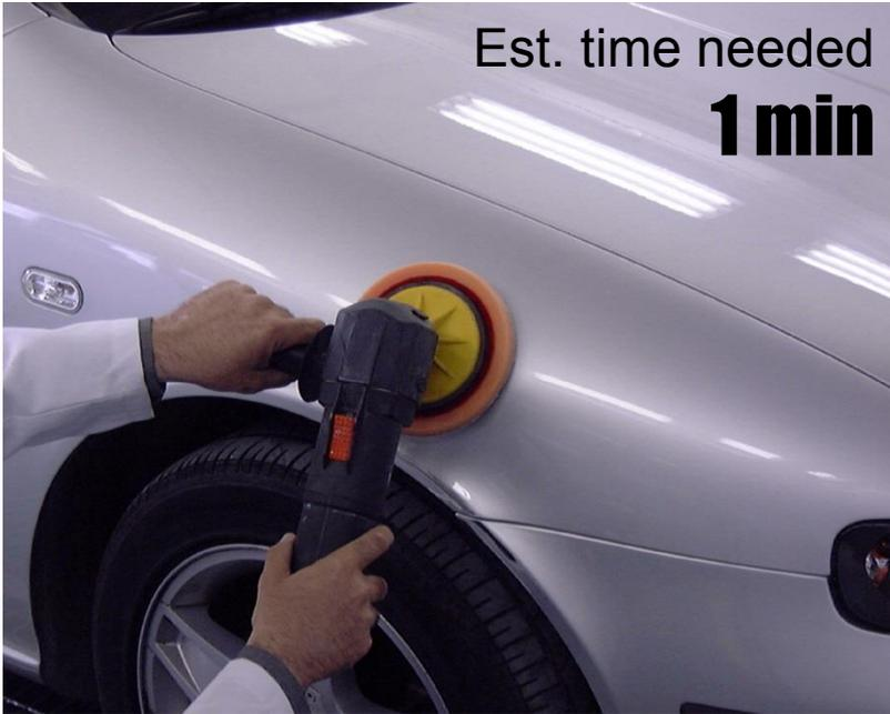
Polish carefully the surface to be repaired to create optimal adhesion
