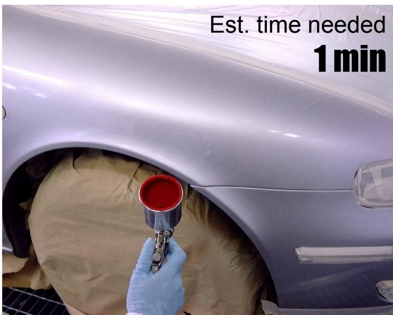
Apply a light coat of the **UV-A1 clear coat** (L19010) thinned at 10% with the **UV-A1 Thinner** (L19007) by Paintgun or by Aerosol (19010)
